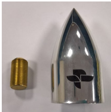
The Articulating claw consists of two pieces; the claw itself and a threaded insert.
