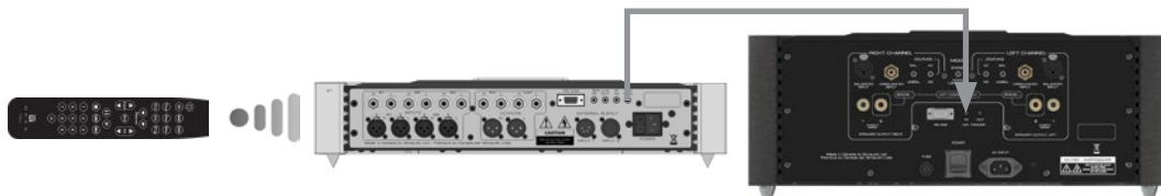
Figure 3: Remote Operation with 12V Trigger
