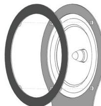
To ensure adequate clearance and prevent damage to the front facia, the grille magnets must locate directly onto the drive unit fixing bolts.
